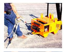
4-part pull Disengage winch and free spool the cable out in order to loop back through the snatch block.
