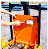
Automatic negative ground switch when door is open light is on, when door is closed light is off.
