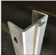
T slot adapter with elongated pin holes
