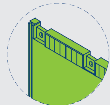
6" Double wall panel with extra heavy duty pounding pad and recessed pull eyes.
